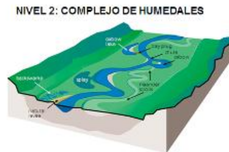
Figure 3.21. Landforms and aspects of a floodplain. Topographic features on the floodplain caused by meandering channels.
