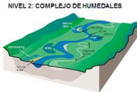
Figure 2.21. Landforms and aspects of a floodplain. Topographic features on the floodplain caused by meandering channels.
